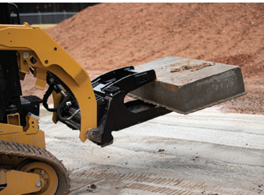
Concrete Slab Bucket
